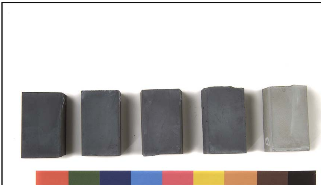
Left to right: Carbocolor® loaded at 6%, 4%, 3%, 2%, and a reference blank.
