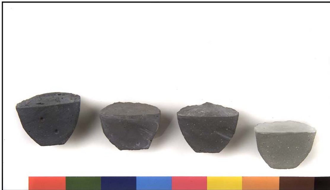
From left to right: Carbocolor®, iron oxide grade A, iron oxide grade B and a reference blank. All coloured samples are loaded at 3% colourant.
